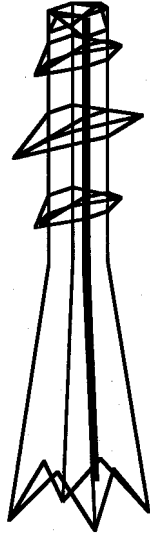
Figure 1—Straight stub on one tower leg
